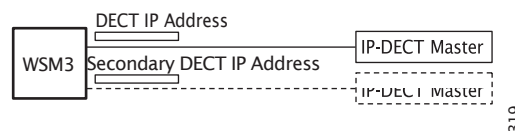
Figure 24. Communication with the IP-DECT system is done over a LAN
